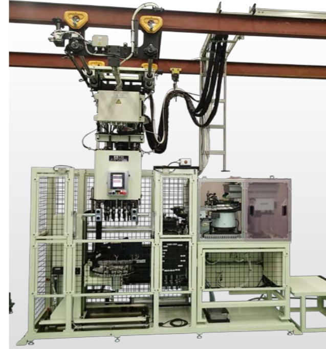
Oil Pan Fastening Machine with Automatic Bolt Feeder
